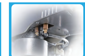
Heating platen pressing & raising speed adjustable by valves
