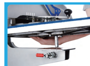
Optional quick-change platens, no tools required
