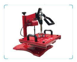
This heat press specifically designed to personalize or customize inflatable youth league sport shoes to professional shoes. Full 360-degree rotation of swing arm allows the heating element to be moved safely aside, reducing the chances of accidental contact. This design is an improvement over clam shell designs.
