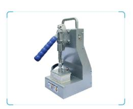
Mini Dual Heat Press is the most compact and lightweight model in our press line weighing in at just 5kg! Despite being small, this manual press generates up to 1000 pounds force. Simply pull the lever and start your label printing . The press features a sturdy construction, a locking lever mechanism, adjustable pressure, 2.5" x 3"(6\*7.5cm) dual heating insulated solid aluminum plates.
