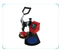
Special designed with digital temperature & timer & alarm for modern fashion pursuing people. Fitting on Diameter 12cm & 15cm plate attachment and make sure working for both small and large plates, Easy parameter setting and the baking time around 180s. Protection with dual electric system to provides safety operation.
