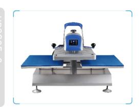
The twin station does twice the work with half the space as a regular swing-away press. One operator can press a job and set another in place. This helps you minimize downtime and keep up with demand, all with one heat press. Besides, LCD screen controller, and live digital time, accurate temperature read-out and Max. 120min set automatic standby.
