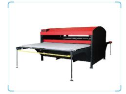
This Industrial Mate heat press is air operated automatic large format twin station shuttle presses that range in platen sizes up to 100 x 120cm standard, and 160 x 240cm for custom i.e. Industrial Mate Max! The B4 is a large format pneumatic heat transfer press built for pressing a wide variety of materials. thicker materials such as carpets & mats, rigid goods like tiles & ceramics.
