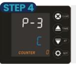
P-3:  $^{\circ}$ C or  $^{\circ}$ F Read-out Touch SET &  $^{\uparrow}$  $^{\downarrow}$  buttons to set  $^{\circ}$ C or  $^{\circ}$ F
