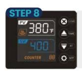
Wake Machine from stand-by You can wake up the heat press from sleepy mode by touching any button on the control panel, and machine starts to heat again.
