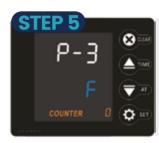
P-3 :  ${}^{\mbox{$\bf C$}}$  or  ${}^{\mbox{$\bf F$}}$  Read-out Touch SET &  ${}^{\mbox{$\bf A$}} \downarrow$  buttons to set  ${}^{\mbox{$\bf C$}}$  or  ${}^{\mbox{$\bf F$}}$
