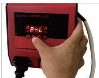
7. Pressing "OK" again and the screen shows "P-L", you need to set a protective temp by press "▼" "▲" (eg.250°F).
