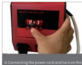
6. Connecting the power cord and turn on the power switch. The display screen should illuminate. Pressing the "OK" key, the screen shows "P-1", you need to set a working temp by press "▼" "▲" (eg.360°F).
