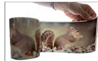
12. Peel off the sublimation paper carefully. A beautiful exclusive mug comes out. Caution: Hot!
