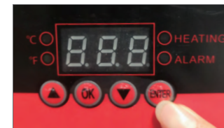
11. When the press raises to the working temp (P-1), it will count down automatically. And it will beep at the end of countdown (display shows 0), reminding you that it's done. Take the mug out first. If you want to sublimate other mugs, please put next one in element, press "Enter" to stop beep, and press "Enter" again to heat up. Otherwise, turn off the machine.
