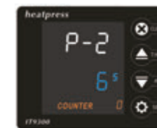
P-2: Time Setting Mode Touch SET & ↑↓ buttons to set desired time.
