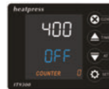
Auto-off Introduction It reads OFF and machine starts to cool down after machine raises to SET temp. and remains no operation for P-4 set time. Operation like control panel setting or heat pressing.
