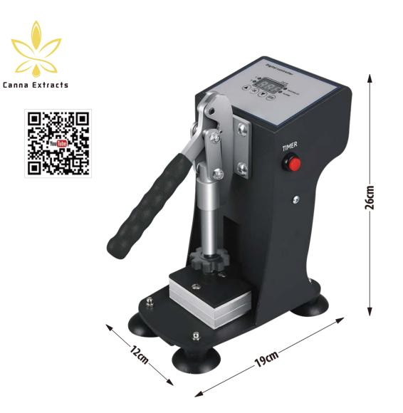
Personal rosin press is the most lightweight model in our press line (G.W. only 4.6kg). Despite being compact, this manual machine generates up to 450kg of pressing force. The press features sturdy construction, a locking lever mechanism, adjustable pressure, 5 x 7.5cm dual heating insulated solid aluminum plates, temperature controls located at the top of the press,. Portable, sturdy and efficient, it is perfect for personal desktop operating or pressing during travel.
